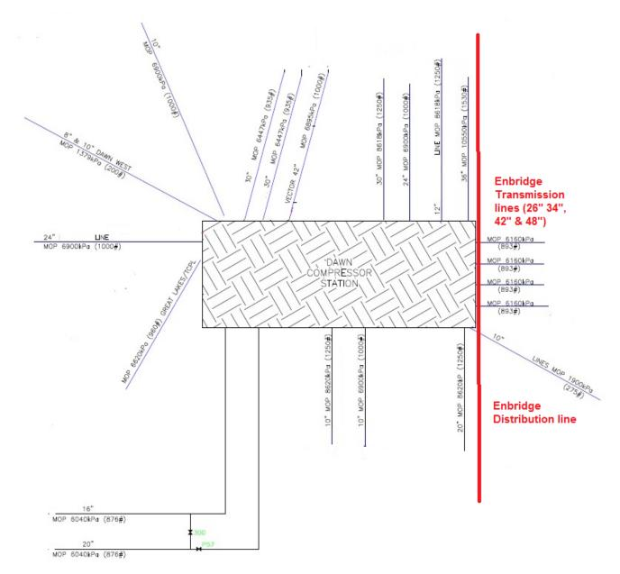
Figure 3: Dawn Pipeline Connections and Pressures
