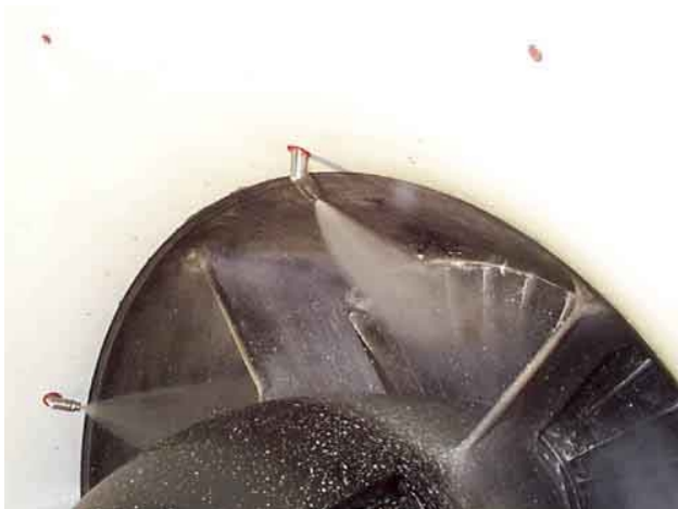
Fig. 2 LM2500 - same nozzles used for crank wash and on-line washing
