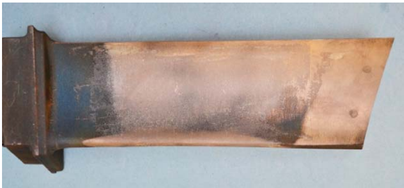
Figure 13: As received condition of the blade. Note the bright surfaces.
