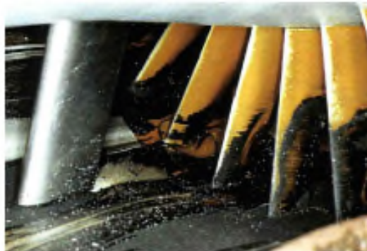
Oil and grease act as "glue" to trap and hold other fouling materials
