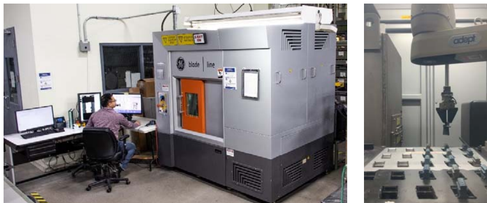
Figure 11 – Bladeline Computed Tomography Machine and Part Holding Bin with Robot Gripper
