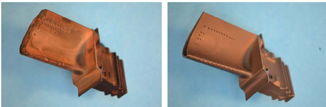
Figure 17 – Post Service (Left) & Fully Repaired (Right) Condition of a GE LM2500 HP1 Blade
