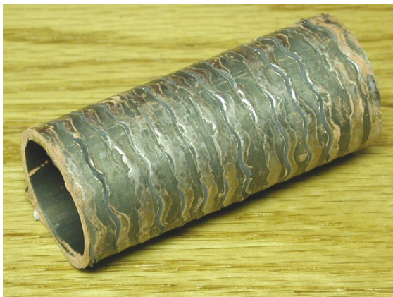
Figure #11 - 409SS fins / SB423 NO8825 after 48 hours
