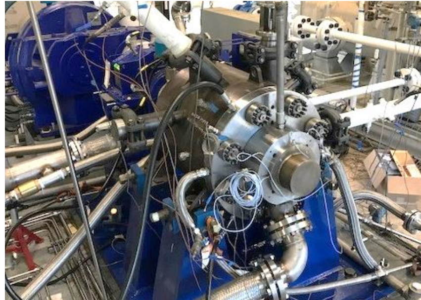
APOLLO 10 MW Centrifugal Compressor 255 bar discharge, full flow test completed in 2021
