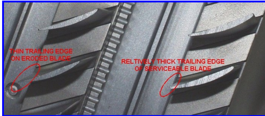
Figure 7: Trailing edge eroded on left compressor blades from exposure to fine dust during operation.
