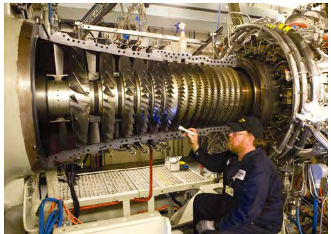
Figure 11. Split Compressor Casing
