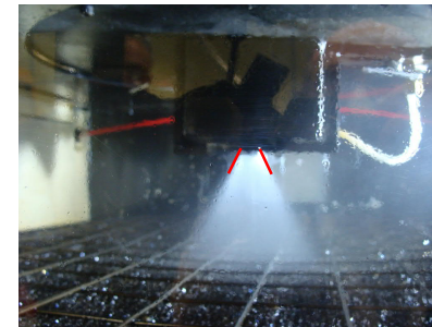
Conventional Dual Fuel Swirler Burner
