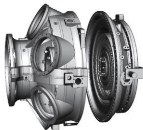
Figure 5: Service friendly compressor turbine module, replaceable in-situ
