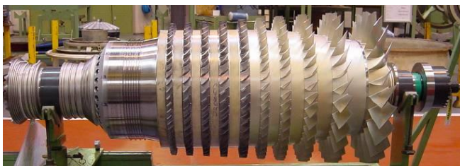
Figure 2a: SGT-300 compressor rotor with high efficient 3D aerofoil design
