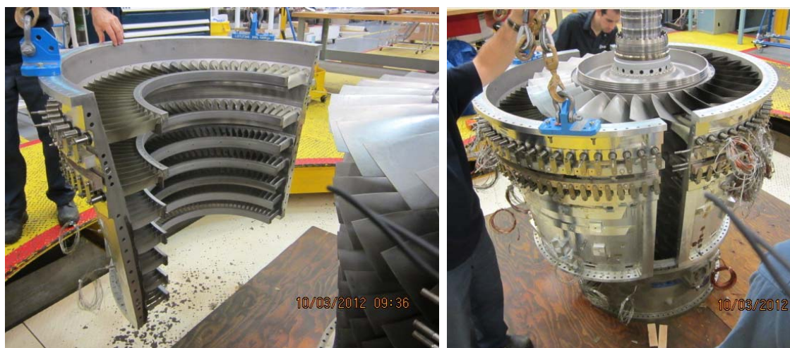
Figure 8: Gzero IPC Casing and stator vanes, and assembly to rotor
