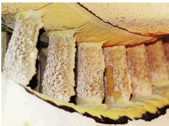
Figure 11: Ash Deposits caused by Crude Oil contamination
