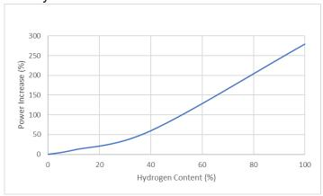
**Figure 16:** Power increase to transport the same amount of energy in a pipeline.
