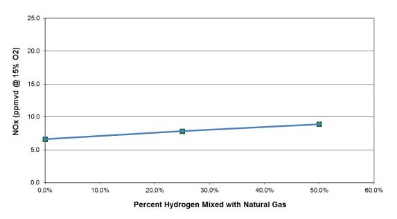
**Figure 8:** NOx Emissions Variation of a 23000hp class gas turbine fuel injector in Combustion Rig Testing at Simulated Full Load Conditions for a 59°F Day and Constant Pilot Level with Varying Blends of Hydrogen Mixed with Natural *Gas*.
