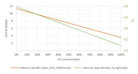
**Figure 9:** The volume calorific value and the mass density at normal conditions depending on the H<sub>2</sub> concentration. The volume calorific value is at normal volume conditions (0 °C and 1 atm) with a reference temperature at 25 °C.
