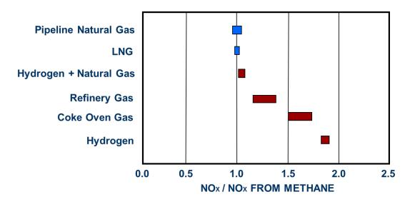
**Figure 4:** NOx Emissions Increase Trends with Conventional Combustion Operating with Hydrogen Rich Fuels Compared to Hydrogen in Natural Gas in the Range of 5 to 20%.
