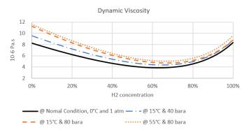
**Figure 11:** Dynamic viscosity depending on the H<sub>2</sub> concentration at different pressure and temperature conditions.
