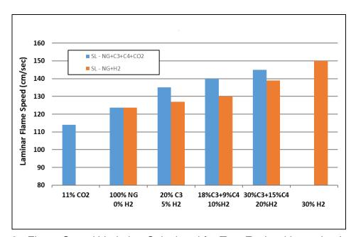
**Figure 6:** Flame Speed Variation Calculated for Test Fuels with varying Levels of Propane, Butane and CO2 Mixed with Natural Gas Compared to Mixtures of Hydrogen and Natural Gas.
