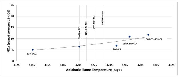
**Figure 7:** NOx Emissions Variation on a 23000hp class Gas Turbine at Full Load and Standard Pilot with Associated Gas Test Fuels with Different Values of Adiabatic Flame Temperature
