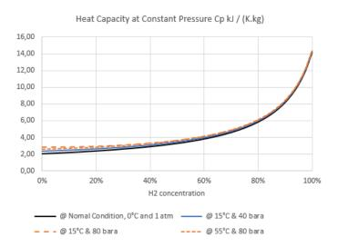
**Figure 12:** Heat capacity at constant pressure depending on the H<sub>2</sub> concentration at different pressure and temperature conditions.
