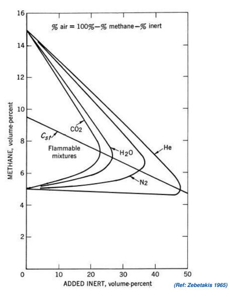
Flammability limits of Various CH4-inert gas-Air mixtures
