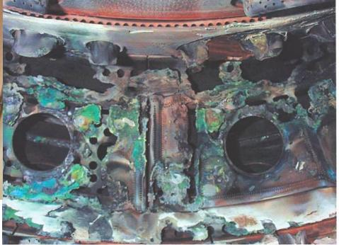
Gas turbines are intolerant to poor "fuel quality"
