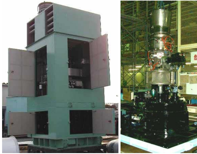
Figure 6. Vertical Pump Package with and without Enclosure
