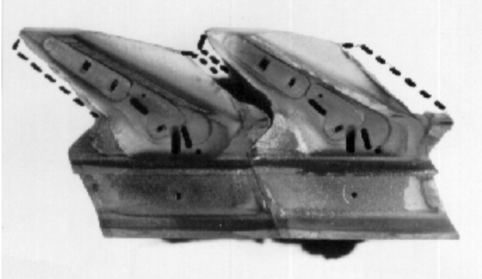
FIGURE 3. Oxidation of RB211 Shrouds
