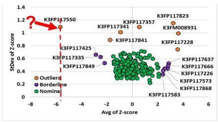
Picture #10: Example of PCRT data plot showing extreme outlier part K3FP117550
