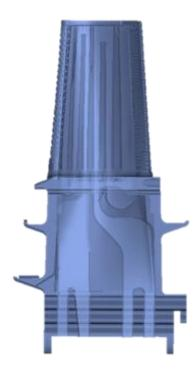
Figure #4: Advanced hot section blades have very sophisticated cooling
