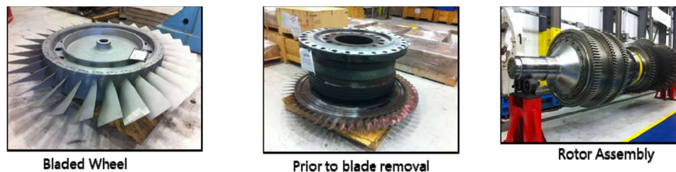
Figure 3: Reverse engineering data gathering of parts and sub-assemblies. Data collected during off-site outage and during on-site rotor overhaul.
