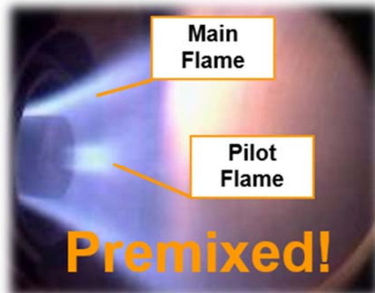
Figure 18: Lean-Premix and Conventional Combustion
