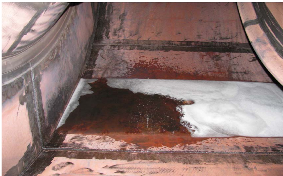
Figure 20: Appreciable amount of wash fluid reaching the exhaust system.
