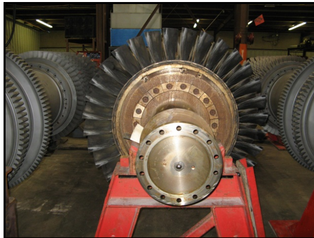
Figure 2. Rotor of GE 5002 Gas Turbine Prior to Overhaul
