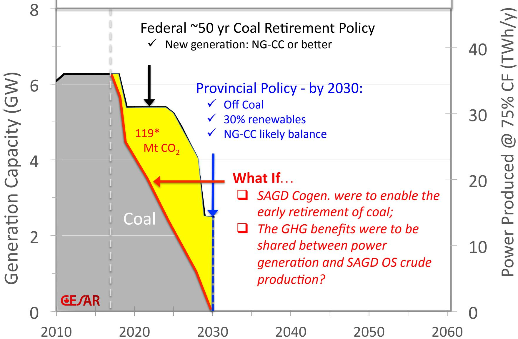
\*Assumes: Coal generation (@ 1008 kg CO<sub>2</sub>/MWh) replaced with NG-Cogen or NG-CC (@ 390 kg CO<sub>2</sub>/MWh)
