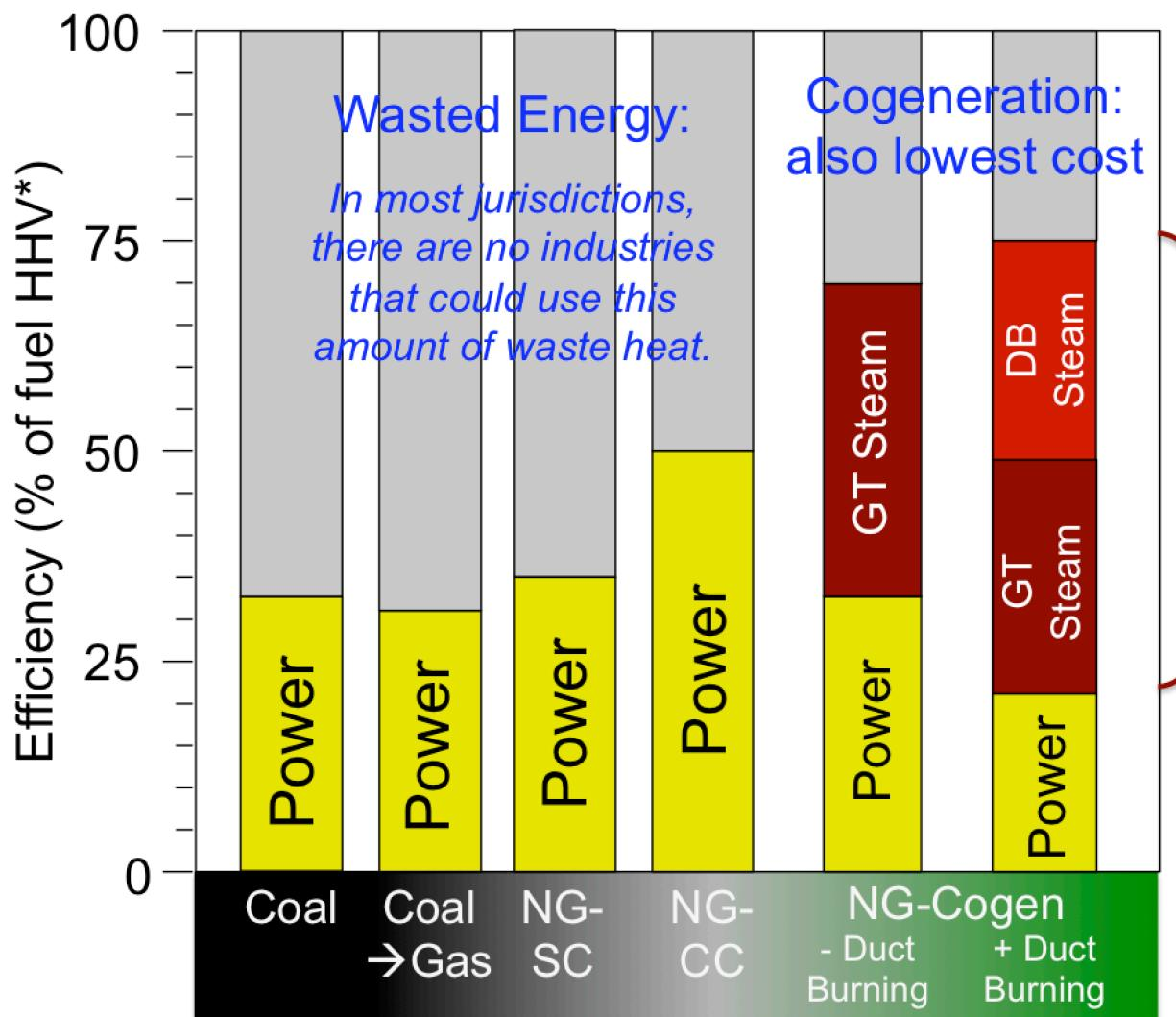
*Cogeneration of heat & power can increase fuel use efficiency to 75% or more if one has an appropriate heat demand.*
