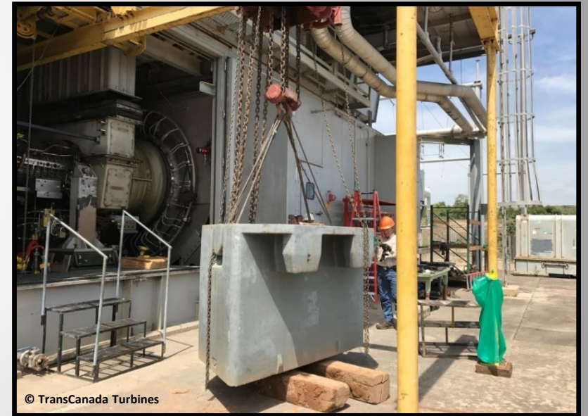
Load Test in Progress of 8.6-ton Chain Hoist and H-Frame
