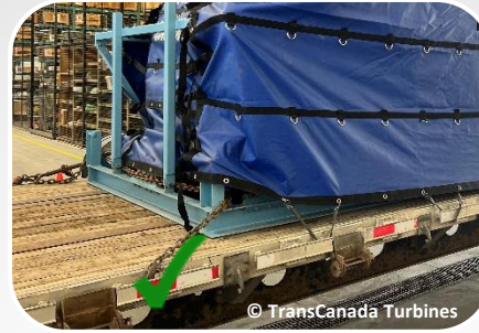
Engines secured with chains
