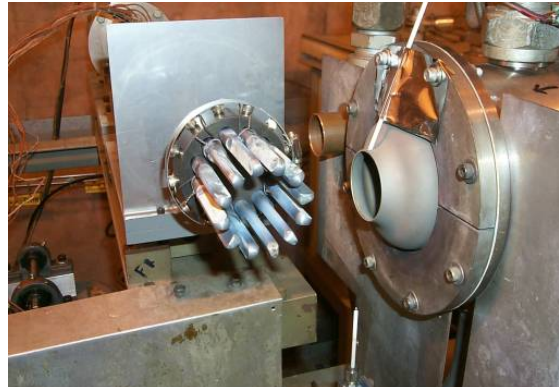
T56 1 st stage nozzle guide vanes
