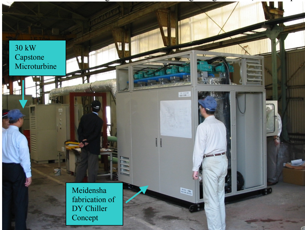
Figure 9 Meidensha 6 bed exhaust gas driven chiller using DY generators, Osaka Japan
