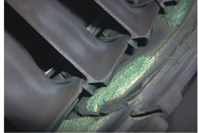
HP Seal Segments showing severe thermal erosion
