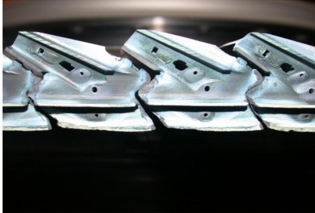
HP turbine blade showing gross erosion of shroud and front seal fin
