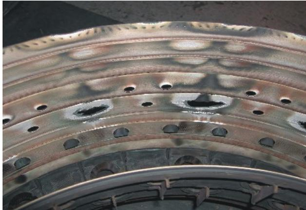
Combustor Outer Wall showing extreme overheating
