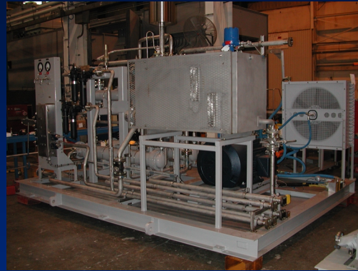
Auxiliary Skid with ~ GLO system ~ TLO System ~ Water Wash System ~ Hydraulic Start
