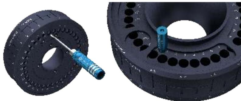
Identify the desired open socket of the mold and install the VPI insert by light pressure. The insert will be able to be installed if only you align the arrow of the insert to the triangular orientation mark of the base. Couple thread the insert to the underside of the mold utilizing the provided VPI Cervico 2mm Allen Screw driver and retention screw.
