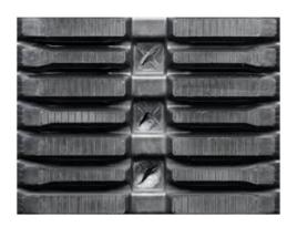
The CTx-MB device will fit the multi-bar track which is popular with the Cat™ CTL machines.
