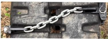
Custom Vortech device can be used straight across or diagonal as shown
