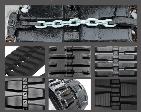
The CTx-SB device will fit the majority of staggered block tracks relative to the above pattern styles.
