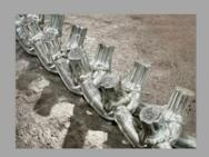
Studded link is ONLY recommended for off-road use. This would be good for forestry applications. We do not recommend this link for gravel/dirt roads due to its aggressive nature.
