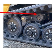
Some of the larger ASV models have no clearance at the Torsion Axle Assembly.
