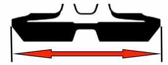
Wrap a stiff wire around the outside edge of the track in the valley and bend the wire around to the underside of the track. We want to see the contour of the track taper.
