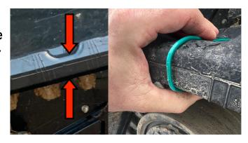
Place the tape measure (as seen below) inside the wire. Keep the butt end of the tape measure inside the upper portion representing the top surface of the track valley. We are capturing the contour of the track to determine the taper of the track thickness.
