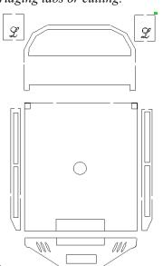
**D:** Determine what truck you are mounting the bed on and set the bed on the frame to determine where you want to apply the Tail Drop. Most beds only have a few inches of overhang so take this into consideration. Apply glue to top of Tail Drop and hold against bottom of Bed until set.
