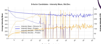
Figure 2: Intensity Mean and Std Dev exhibit good separation values for Intensity Mean and are higher for protein than silicone oil.
