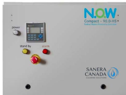
The Radical Waters N.O.W single stream High salt ECA Generators use a single cell (or multiple cells in series and parallel for larger generator configurations). Brine flows through both the anodic and cathodic chambers. The Anolyte pH is controlled by adding Catholyte to the anolyte. Excess Catholyte is directed to drain but can be collected and used as a detergent. This configuration uses 0.4 – 0.5% brine solution as the precursor.
