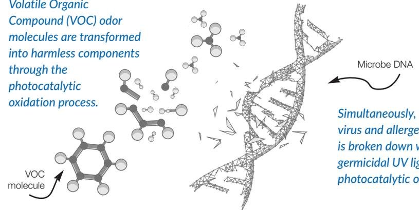
Simultaneously, bacteria, virus and allergen DNA is broken down with germicidal UV light and photocatalytic oxidation.
