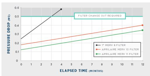
Aprilaire filters, with over nine times the surface area, have extremely low initial resistance and high dust holding capacity, allowing them to work for 12 months without being overly restrictive. This helps maintain proper airflow, reducing potential call backs.
