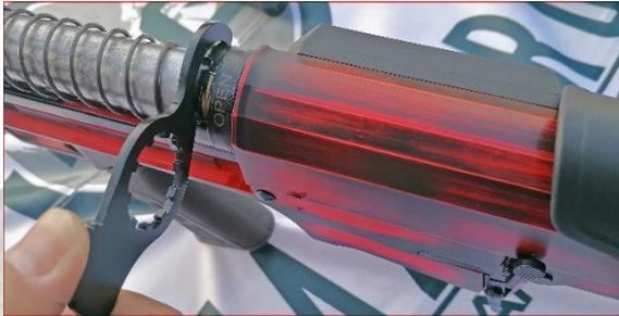
12. Remove the arm by pulling the mainspring inside the mechanism.
