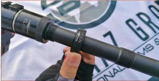
7. Remove the Gas Chamber by Turing it counter-clockwise.
