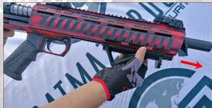
5. Remove the charging Handle, by taking it out from the left or right side of receiver and take out the handguard but pushing it forward.
