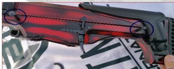
7. Fix the handguard by pushing it backward direction.
