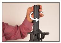
**3)** Take out the Muzzle Brake by turning counterclockwise
