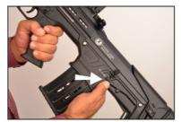
2) Use the Magazine Plug on the right side of the firearm or use the Magazine Catch on the left side of the firearm to take out the Magazine
