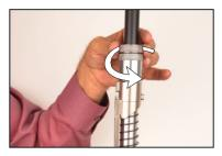
**9)** Take out the Gas Block Adjust Screw by turning counterclockwise and take out the Gas Block by turning clockwise
