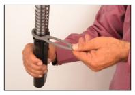
**10)** Take out the Barrel Assembly Nut by turning counterclockwise
