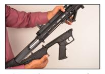
**7)** Separate the Upper Receiver from the Lower Receiver
