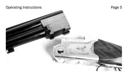
Swing the barrel up firmly without forcing to its fully closed position. The lever will snap to a centered position. The barreled action is now ready to receive the forearm.
