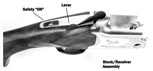
The stock/receiver is now ready to accept the barrel assembly. To assemble the barrel to the stock/receiver assembly, locate the half-round cuts in the barrel lug and the round hinge pins inside of the receiver. With the barrel assembly held approximately 45 degrees to the stock/receiver assembly, mate the round cuts of the barrel assembly to pivot on the round receiver hinge pins.
