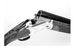
Inspect the bore and chamber for excess oil, grease or other obstructions. (The chamber is the rear portion of the barrels where the cartridges will be inserted.) You can now close the firearm to check for binding. You may want to repeat opening and closing the firearm several times to become familiar with its function, and to ensure that it is properly assembled.
