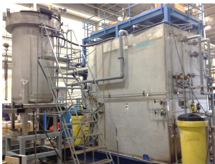
Figure 2. Pilot system PACT MBR setup.
