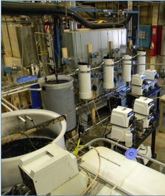
Figure 1. Flow-through bench PACT MBR setup.
