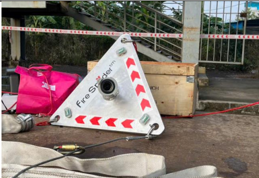
Photo 03. The triangle plate with quick coupling and nozzle that will be winched to the fire floor to fight the fire.
