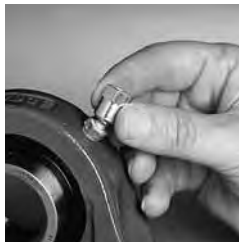
2. Place a Zerk-Lock onto the fitting
