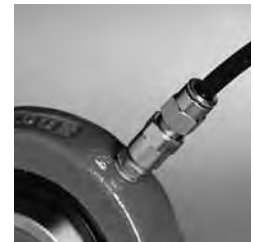
5. And plug the tube into the Quickline adapter
