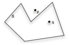
If there is a straight line across the point and the polygon that have odd intersections with the polygon, then the point is inside the polygon. Otherwise, outside.
