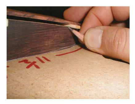
12. Lining up the centerlines again and mark the edges of sides to the braces using a cut off pencil tip.
