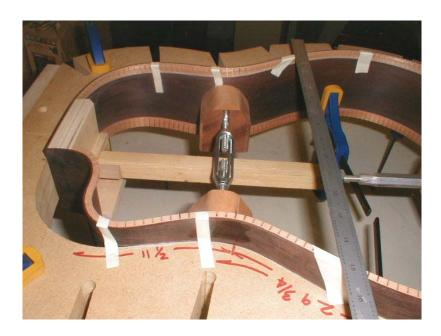
8. Remove the camps and pop off the back. Voila! You have just transferred the exact brace pattern to the sides...ready for notching.
