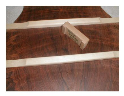
1. Start by deciding how tall you want the scalloped portion of the braces to be. I have seen from almost-no-height to 1/8" or more. I use a nominal .100" tall. This height dimension is cut into a block of MDF with a Dremel in order to create a channel to hold a strip of sandpaper. The block size is not critical but one should keep in mind that this block mostly acts as a sander, so make it comfortable to hold in your hand.
