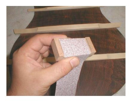
2. Cut a strip of 100 grit abrasive that match the width of your notch in you sanding block. Note that the braces are left "long".
