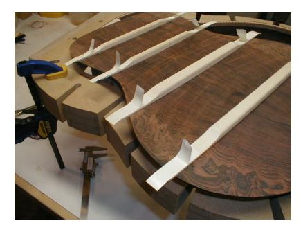
5. Apply the strips of tape on the ends of the braces and remove the protective backing.
