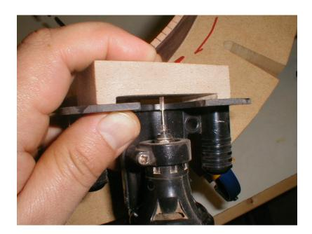
10. Start the notching process by establishing the notch height by placing your Dremel router bit (I use a 3/32" dental burr) into the sandpaper notch of your block. This establishes the notch height for your lining to receive your braces perfectly.
