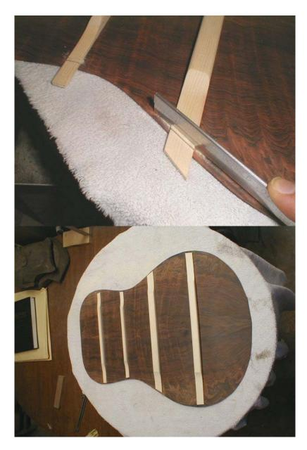
14. Cut the excess portion of the braces off and prepare the back for gluing and test fit the back to the sides - most often there is little to no tweaking necessary.
