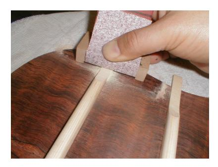
3. Sand the end of each brace until you can sand no more. As you can see, this establishes a consistent brace end height. With the grain of the wood clean up the rough sand line to 220 grit by hand.
