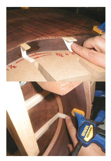
7. Now begin to peel back the tape from the brace ends and stick it to the sides of the guitar. This is repeated inside the guitar.
