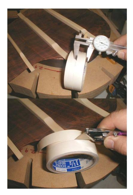
4. Using thin double-sided tape, begin to cut strips that are the exact width as your braces. I use calipers to measure, and scribe to the roll of tape. Once marked, I use a razor to cut the individual strips of tape. The strips should be around 3" long or so. Don't make the strips too short because thy will be too difficult to work with for the next step.
