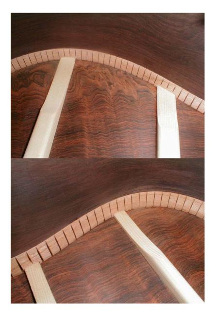
15. Glue the back to the sides and clean up any glue squeeze out around the lining with water and a bristle brush. You should now have perfectly notched lining without weird gaps or funkiness. Whew- maybe some day I'll make a fixture.
