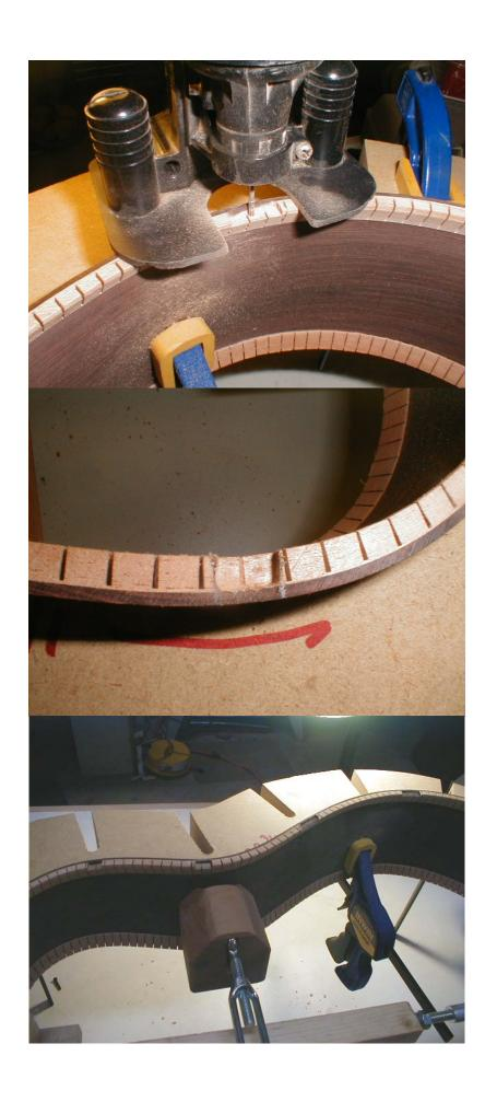
11. Simply route out the brace portion in the lining being careful not cut outside the lines.
