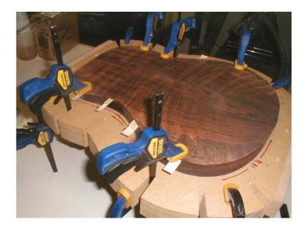
6. Now carefully position the back to the sides, aligning the center points for the final fit of the back and throw on a few clamps to hold it down and in perfect position.
