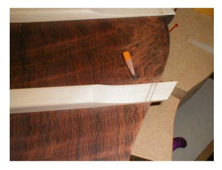
13. Transfer the thickness of the sides of the guitar to the recently marked side profile. Remember to add a little to this dimension for expansion of the braces over time.
