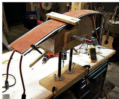
For the process, I use two blankets, one on the top and one below, bending both sides at the same time. I also use two 6" x 36" pieces of thin and flexible stainless steel between the wood and silicone blankets, making a side sandwich with a total of six layers.
