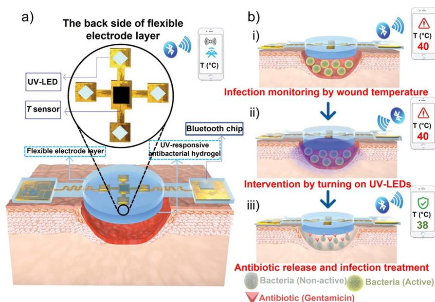
**Figure 8.** Sensors for wound environmental parameters. a) Construction and working principle of an intelligent dressing, incorporating flexible electronics for wound monitoring. b) Integrated system for monitoring wounds infected with bacteria. (a) and (b) Adapted with permission from ref. [79]. Copyright 2020 Wiley Online Library.
