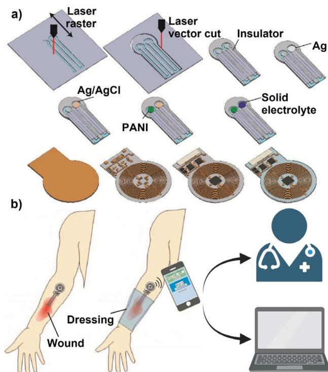
**Figure 6.** Sensors for wound environmental parameters: a) Fabrication of a pH sensor on an ITO electrode. b) Schematic of the integrated and flexible NFC communication system for measuring wound pH. (a) and (b) Adapted with permission from ref. [72]. Copyright 2018 Elsevier.
