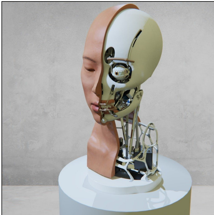
Figure 12: CAD model of the skin and skull (Rendered in Keyshot)
