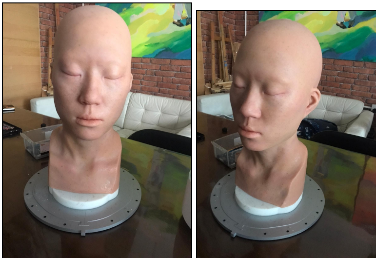
Figures 10&11: Physical model of the silicone skin of the head.
