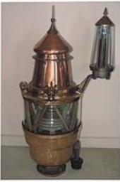
Buoy light with sun valve.
