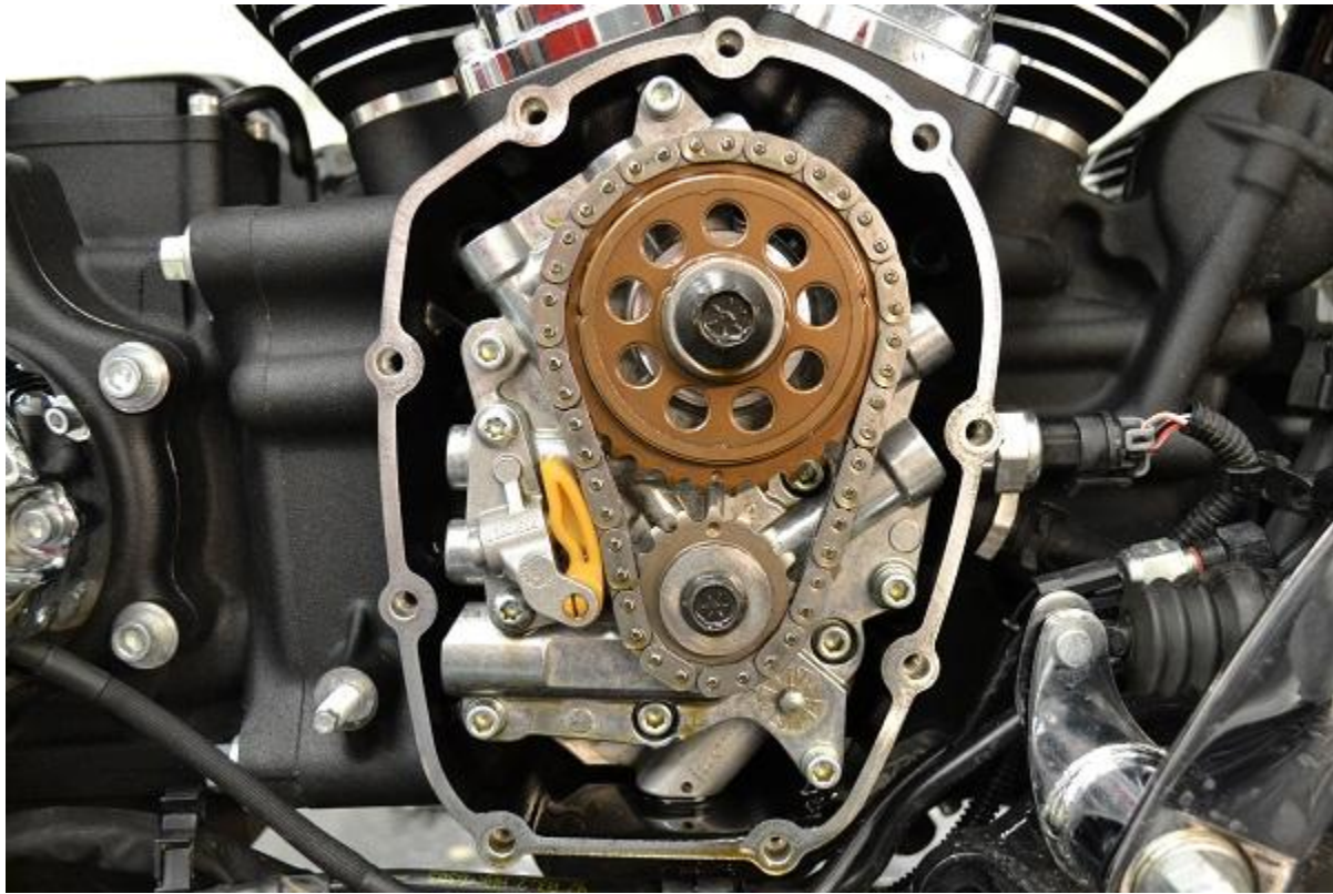
camchest with cam plate removed
